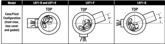
NOTE: Switches shown tripped on falling level.
